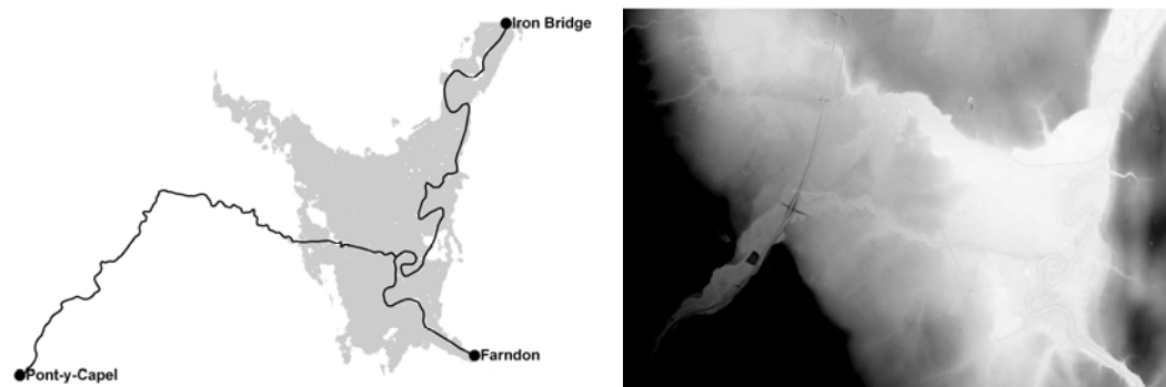
Figure 3: Test site: River Dee between Farndon and Iron Bridge and River Alun between Pont-y-Capel and the confluence (black line); Environment Agency gauging stations (black circles); flood extent derived by using the ESA satellite image (ERS-2 SAR, grey area) [left panel]; DTM at 2 m resolution derived by using LiDAR and IfSAR data (grey scale) [right panel].
