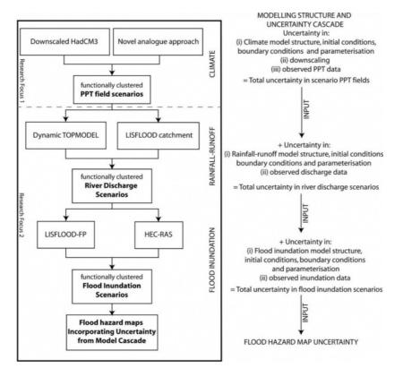
Figure 6. Modelling structure and uncertainty cascade in the project aimed at assessing uncertainty in flood inundation impacts (courtesy H. Cloke).
